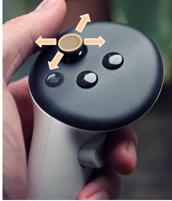
(b) Left controller mapping: thumbstick controls the polar angle.
